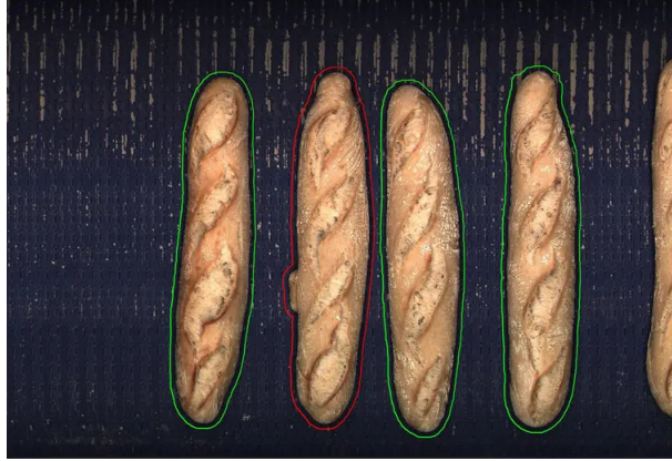
Figure 5: This picture shows an in-production use of anomaly image detection. Image from MVTec [2024].
